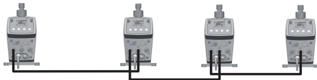
Fig. 14: Synchronization of several dosing pumps by means of stroke feedback and pulse control
